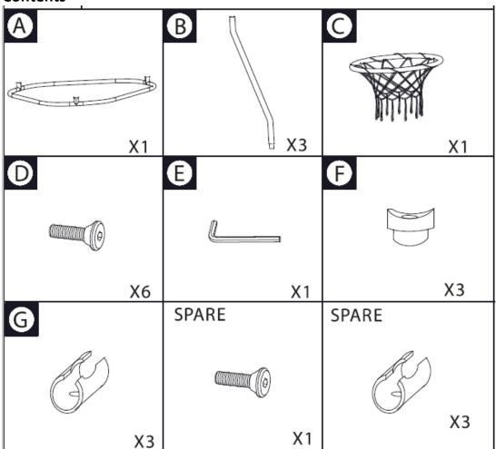
Fit the 3 legs (B) to base (A) using 3 bolts (D). Clip the 3 plastic feet (G) to base (A).
