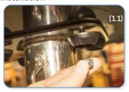
1. Attach the steel legs to the base of the instrument with the M8 Nyloc Nuts and 2 part security caps. (1.1) (See Assembly Guide)
