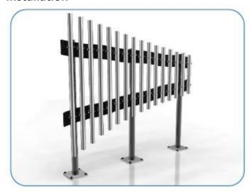
1. Carefully lay 3 x legs on a level surface and check distance between each leg is equal. Join together the 2 parts of the symphony. Line up pre drilled holes in the backboards with the legs and ensure the instrument is aligned square with the legs. Fix in place using M8x40mm screws supplied (see installation guide)
