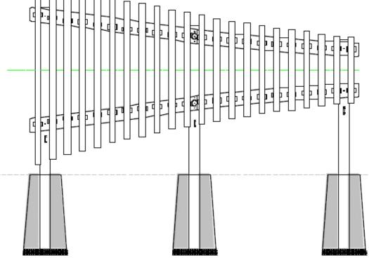
Fill holes with fast drying concrete to manufacturers specifications. If posts protrude above instrument they can be cut down
