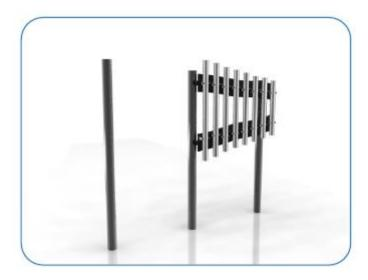
3. Carefully raise the instrument from the ground with legs attached and locate (lower) legs into holes making sure they are vertical and level prior to concreting in place.
