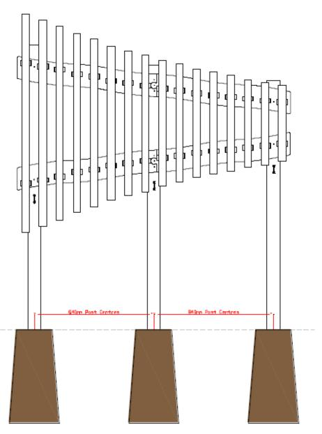
2 Excavate 3 holes with a 250mm diameter tapering down to 350mm diameter and 650mm depth
