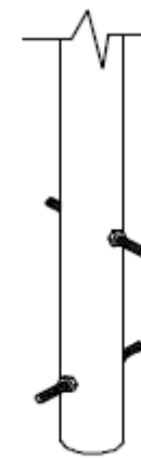
2 Fix M10x 150 Threaded bar in place using M10 Nuts
