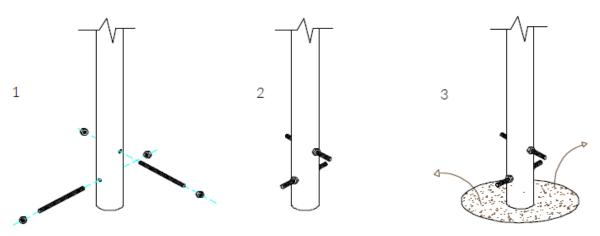
Insert M10x 200 Threaded bar into pre drilled holes in Ground Fixing Post
