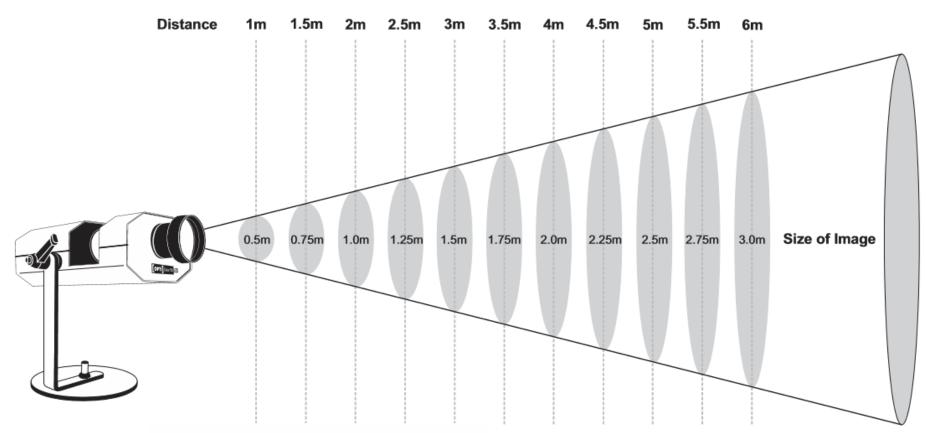
85mm (Lens) Ratio for Distance 2:1 (Image Size - 85mm Lens) The Object Diameter is 42mm
