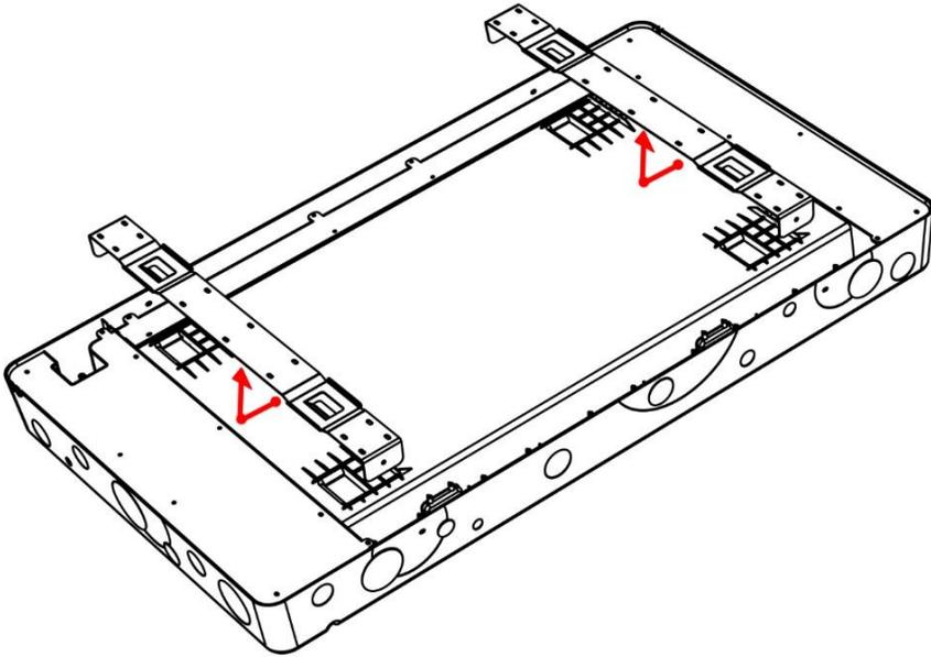
3. Hold the panel where you would like it to be mounted ensuring it is level. Whilst in position mark where the centre of the bracket mounting holes are on the wall. Do this for all 4x bracket mounting holes.
